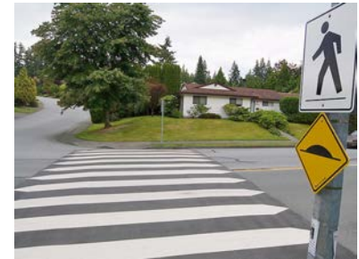
Raised crossings can be distinguished from the street through a variety of painted markings or surface treatments. They can be simply designed on neighborhood streets or a more formally designed streetscape element in a downtown setting.
