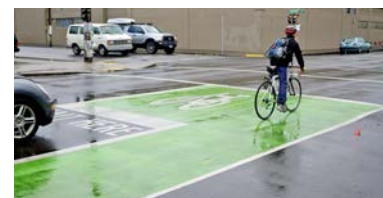
Green paint can be used to distinguish bike lanes from vehicle travel lanes, particularly in locations with heavy traffic. This intersection also has a 'bike box' delineated, which is a space for bicyclists waiting for the light to turn or travel through the intersection with traffic. Vehicles are stopped behind the bike box.
