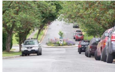
A small, simple roundabout at the intersection of two neighborhood streets.
