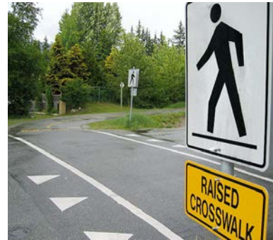
Raised crossings can be distinguished from the street through a variety of painted markings or surface treatments. They can be simply designed on neighborhood streets or a more formally designed streetscape element in a downtown setting.
