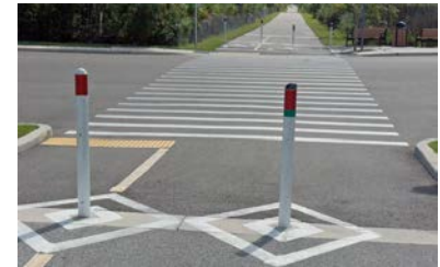
Shared-use path crossing a street. Pedestrians should cross on the left and bicyclists on the right. Bollards separate the path and street.
