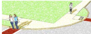
Combined curb ramps.
